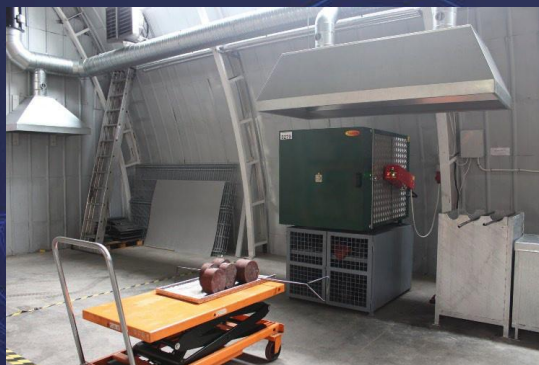
Furnace KPM120/1200 for quenching and tempering of parts
